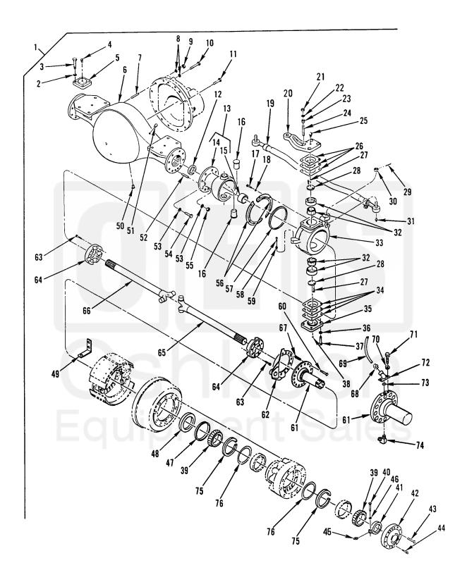
Figure 178. Front Axle Assembly (M916A1, M916A2, M917A1's)
